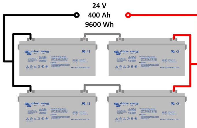
Four batteries in series/parallel
