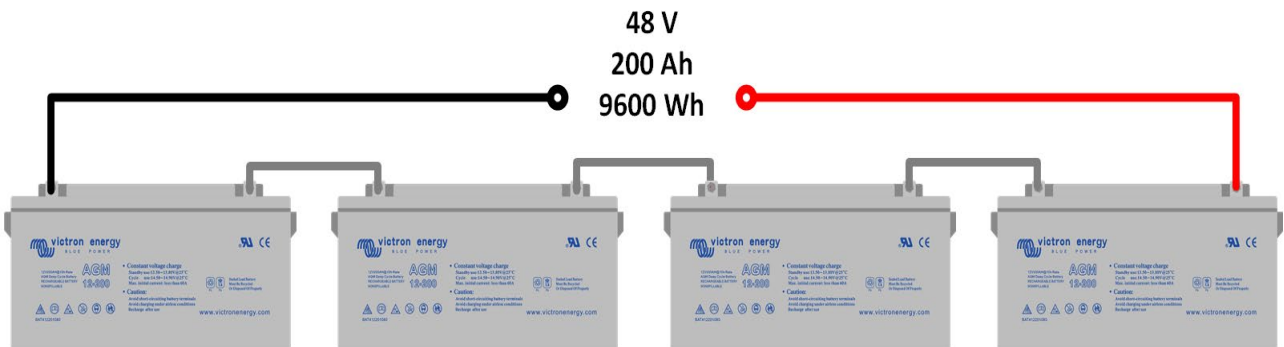
Four batteries in series
