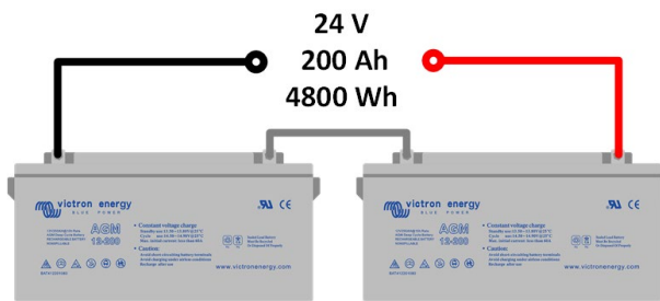
Two batteries in series
