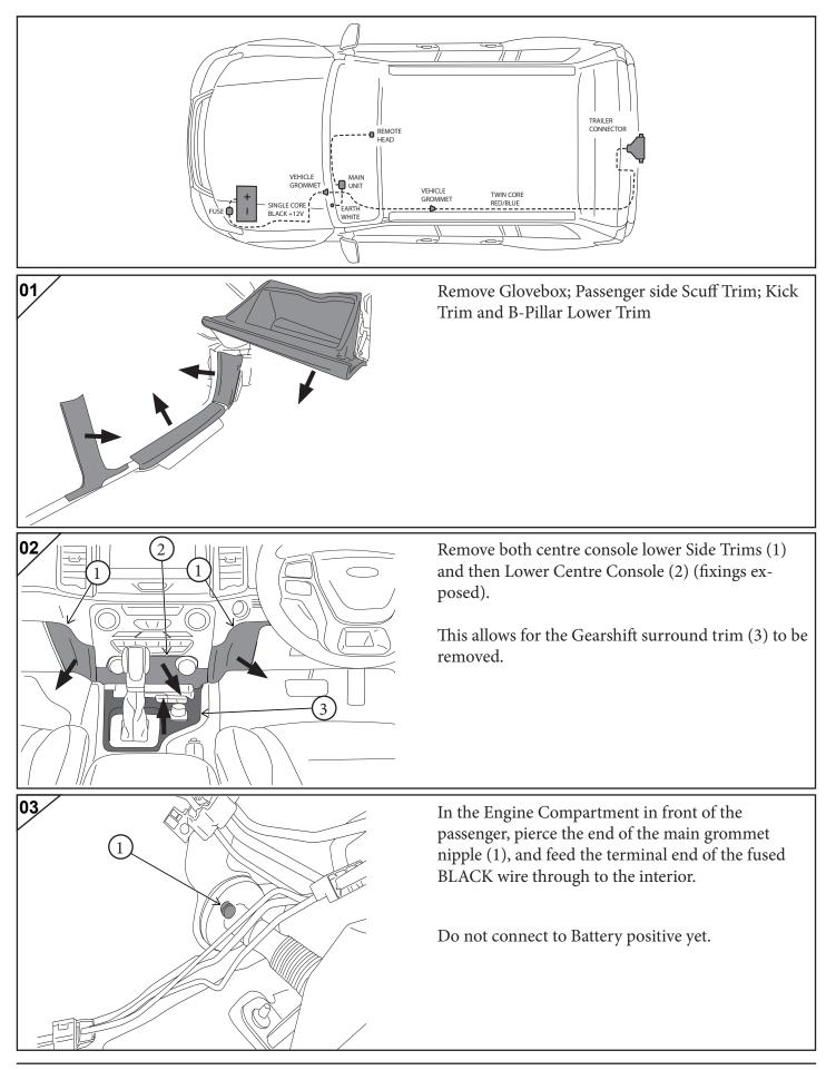
Electric Trailer Brake Controller Kit fitting instructions, suitable for:
