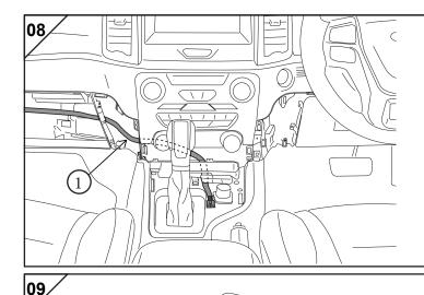
Route the Remote Head cable (1) along existing wiring (forward of glovebox hinge) to the area to the Right Hand Side of the Gear shift.
