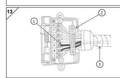
If any BLUE is fitted to terminal 5 position, remove and insulate, pulling back to main harness.
