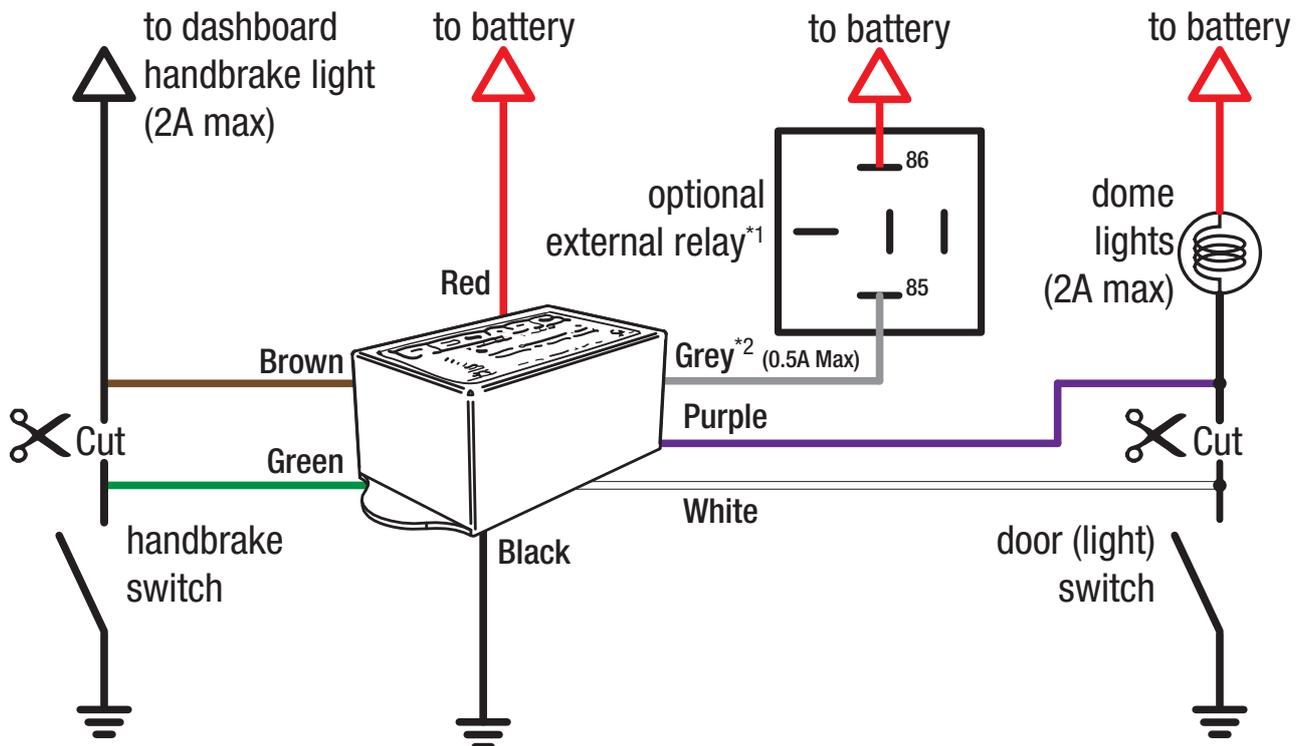
Please note that a combination of the two wiring diagrams may be used to suit vehicles with either positive door and negative handbrake switches, or negative door and positive handbrake switches.
