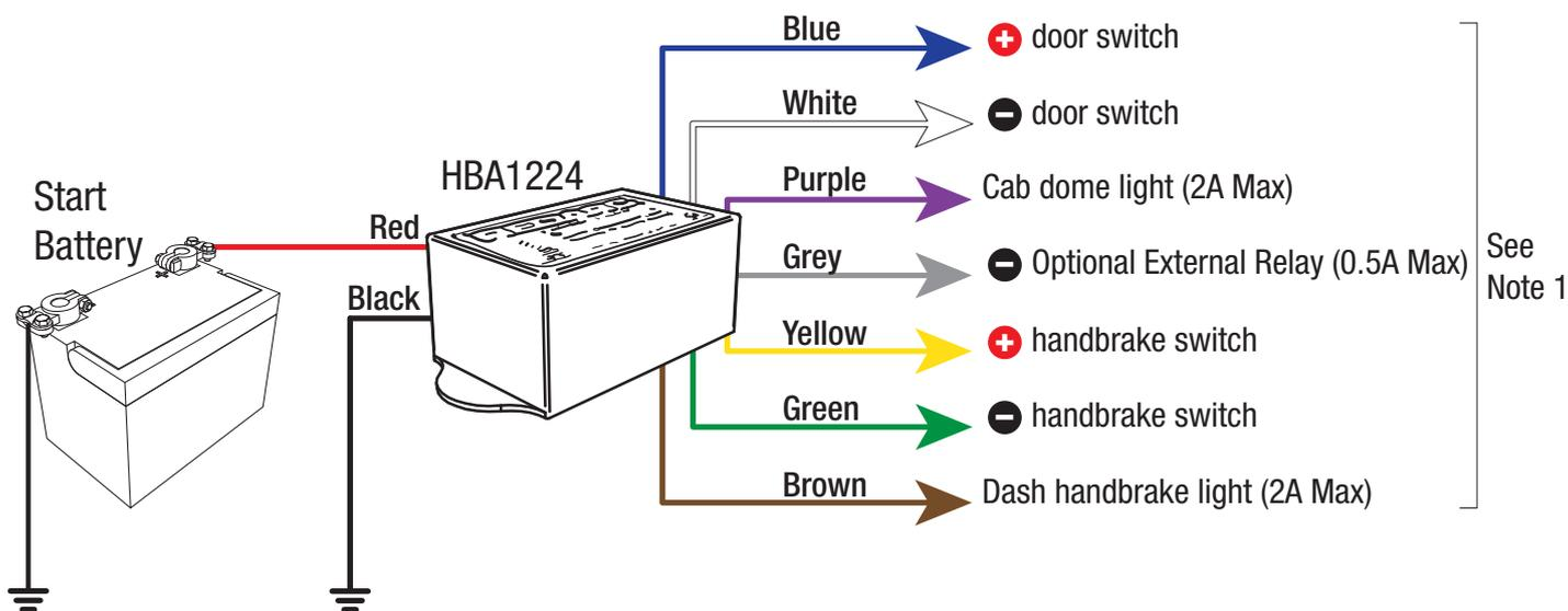
The Handbrake Negative input (Green wire) has specific operating voltage requirements. Care should be taken if other circuits, electronic controls or power circuits are connected to this input which may cause voltages other than battery positive or negative. The following specification applies:
